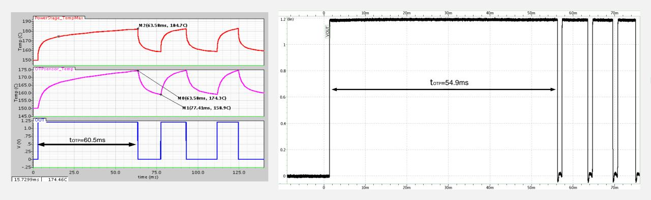
> Good agreement between the measurements and the electro-thermal simulations results regarding the time until the OTP event occurs ( $t_{OTP}$ ): 59.5 ms and 60.5 ms
